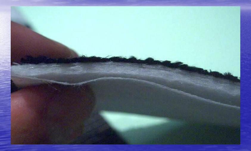
**TECASORBmade of elastic fibres** with macroscopically smooth surface made of hydrated cellulose fibre Thermally processed fibre Specialised technology outcome with higher temperatures -> material made of activated carbon fibres with high absorbance
